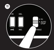
When the record is finished, the **Tonearm** will automatically stop (if set to **AUTOSTOP**). Lift the **Tonearm** from the record and return it to the resting position. If set to **DJ**, the **Platter** will keep rotating. To stop manually, lift the **Tonearm** from the record and return it to the rest.
