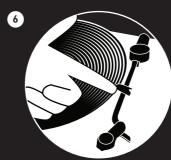
Release the **Tonearm Lock,** and remove the protective cap from the stylus.
